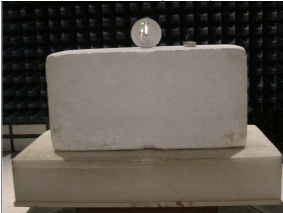
Radiated Emission Test (Above 1GHz)
