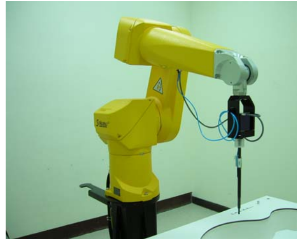
Fig. 5.2 Probe Setup on Robot
