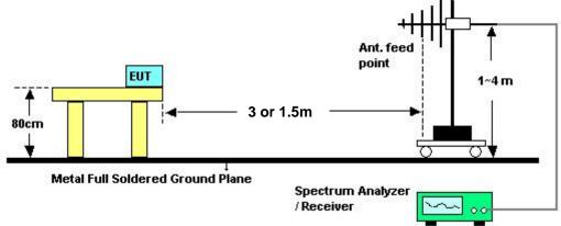
Above 10 GHz shall be extrapolated to the specified distance using an extrapolation factor of 20 dB/decade form 3m to 1.5m.
