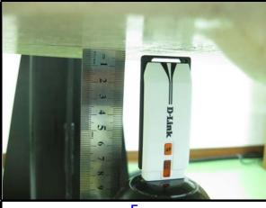
The tip of the EUT faces to the phantom with 5mm-separation distance.
