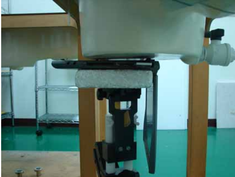
Fig. 9.5 DELL PP03L Notebook Bottom Touch with Horizontal USB Port
