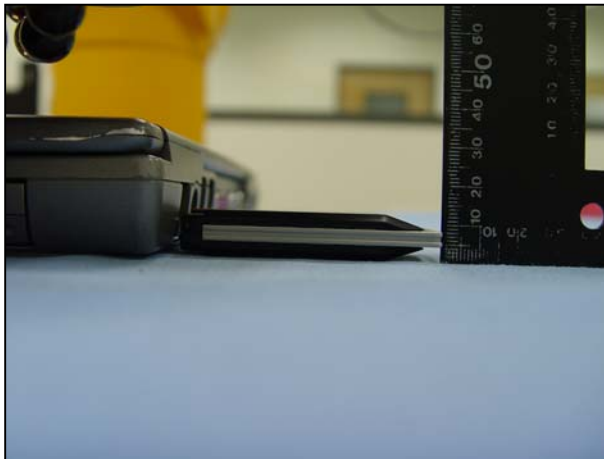
Distance is 1mm for Bottom Face Touch
