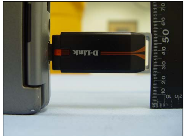
Distance is 25mm for Side(Edge)Touch
