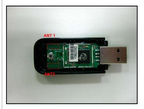
**NOTE:** Only antenna 1 can transmit under 1TX mode.
