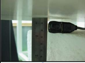
The left edge of the EUT faces to the phantom with 5mm-separation distance.
