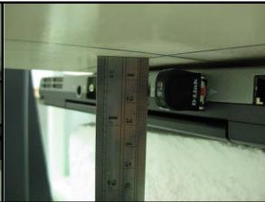
The right edge of the EUT faces to the phantom with 5mm-separation distance.
