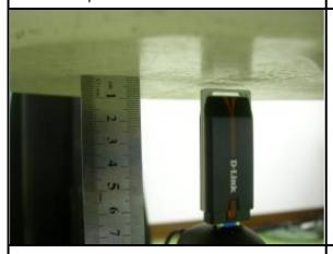
E: The top of the EUT face to the phantom with 5mm-separation distance.
