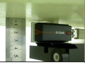
**D:** The right of the EUT face to the phantom with 5mm-separation distance.
