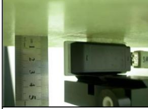
**C:** The left of the EUT face to the phantom with 5mm-separation distance.
