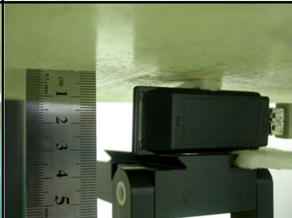
D: The left edge of the EUT face to the phantom with 5mm-separation distance.
