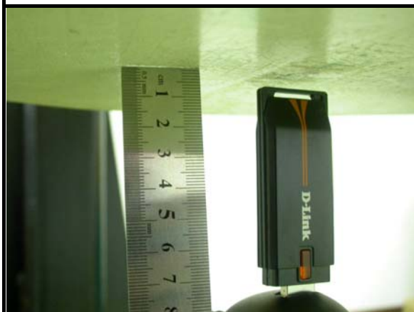
E: The top of the EUT face to the phantom with 5mm-separation distance.
