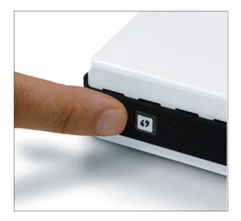
Press the WPS button on the adapter and holding for two seconds until the utility screen comes up. Then, press the WPS button on the router/access point to continue.
