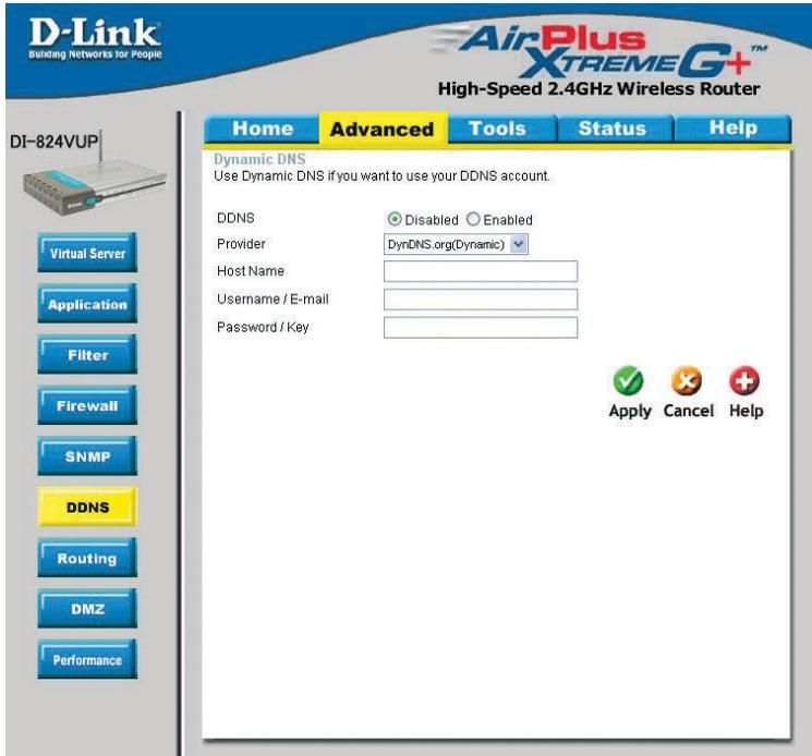
DDNS (Dynamic Domain Name System) keeps dynamic IP addresses (e.g., IP addresses assigned by a DHCP capable router or server) linked to a domain name. Users who have a Dynamic DNS account may use this feature on the DI-824VUP.
