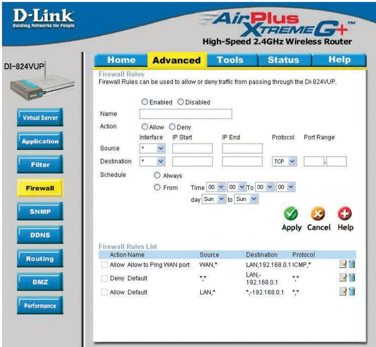
Firewall Rules is an advance feature used to allow or deny traffic from passing through the device. It works in the same way as IP Filters with additional settings. You can create more detailed rules for the device.
