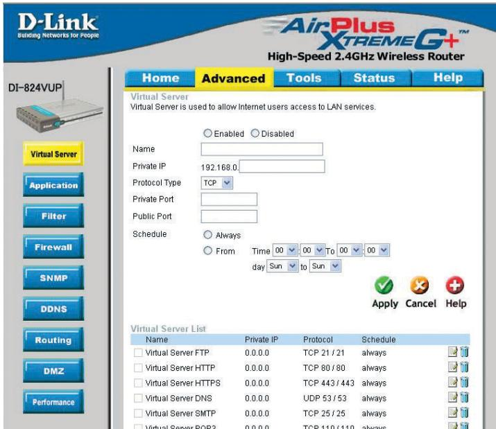
The DI-824VUP can be configured as a virtual server so that remote users accessing Web or FTP services via the public IP address can be automatically redirected to local servers in the LAN (Local Area Network).
