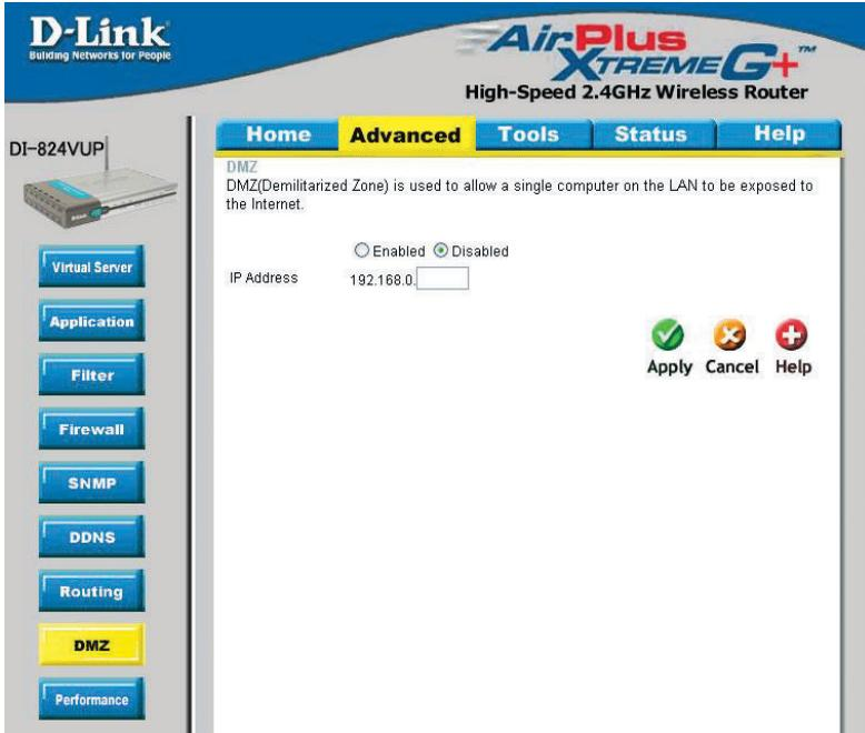
If you have a computer that cannot run Internet applications properly from behind the DI-824VUP, then you can allow that computer to have unrestricted Internet access. Enter the IP address of that computer as a DMZ (Demilitarized Zone) host with unrestricted Internet access. Adding a client to the DMZ may expose that computer to a variety of security risks; so only use this option as a last resort.
