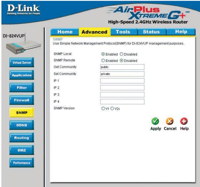
SNMP (Simple Network Management Protocol) is a widely used network monitoring and control protocol that reports activity on each network device to the administrator of the network. SNMP can be used to monitor traffic and statistics of the DI-824VUP. The DI-824VUP supports SNMP v1 or v2c.
