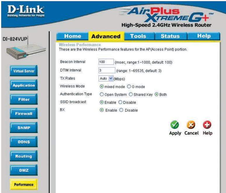
**Beacon Interval** Beacons are packets sent by an Access Point to synchronize a wireless network. Specify a value. **100** is the default setting and is recommended.
