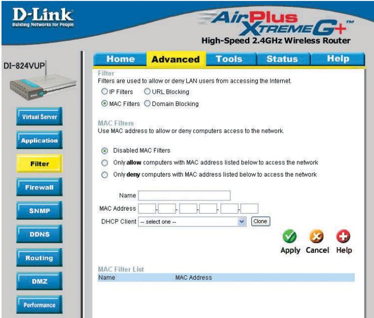
MAC (Media Access Control) Filters are used to allow or deny LAN (Local Area Network) computers from accessing the Internet and network by their MAC address.
