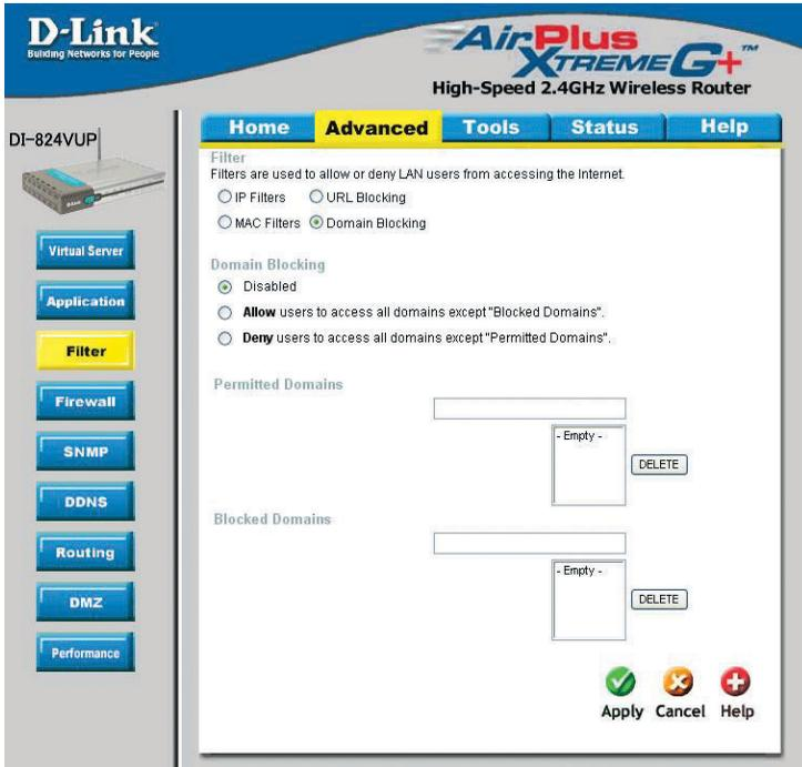
Use Domain Blocking to allow or deny computers access to specific Internet domains whether it is through www, ftp, snmp, etc.
