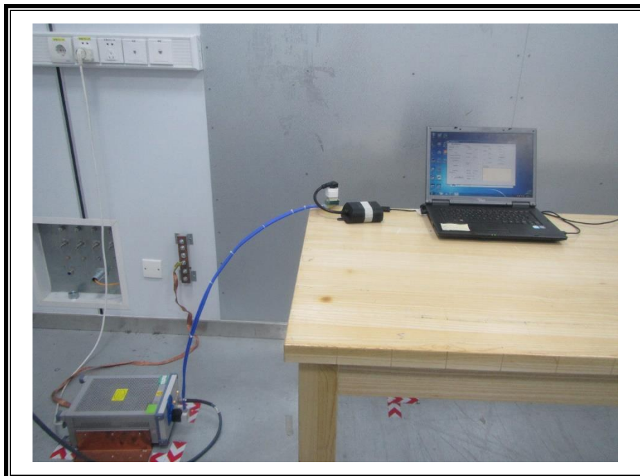
POWERLINE CONDUCTED EMISSIONS MEASUREMENT SETUP
