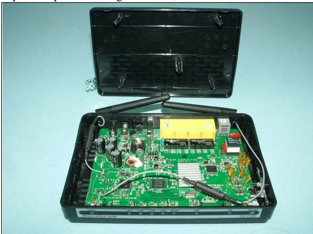
Sample 3: Dipole antenna gain is 2dBi, Antenna connector is soldering
