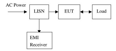
The EUT are connected to the main power through a line impedance stabilization network (LISN). This provides a 50 ohm/50uH coupling impedance for the measuring equipment. The peripheral devices are also connected to the main power through a LISN that provides a 50ohm/50uH coupling impedance with 50ohm termination.
