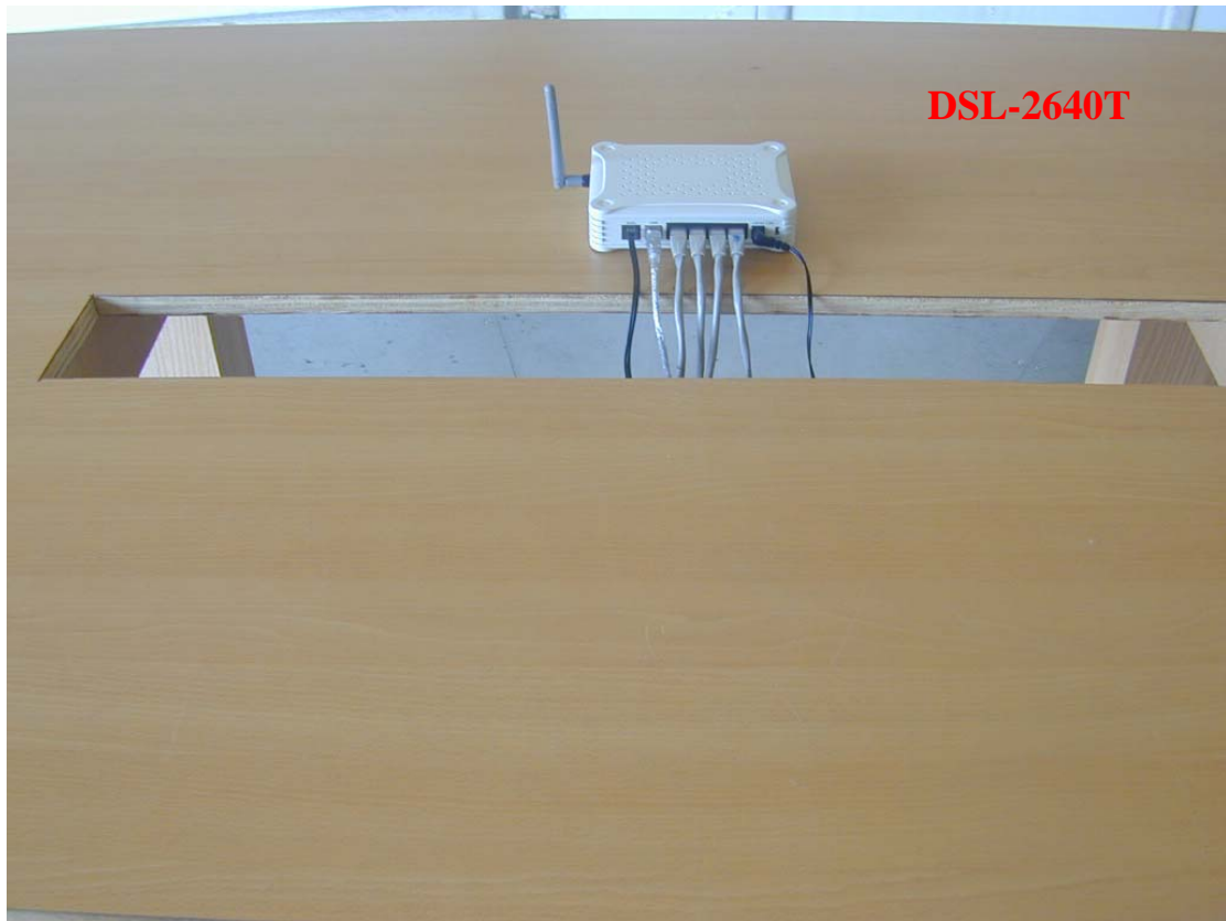
Photo 1: Radiated Emission Test Set-up
