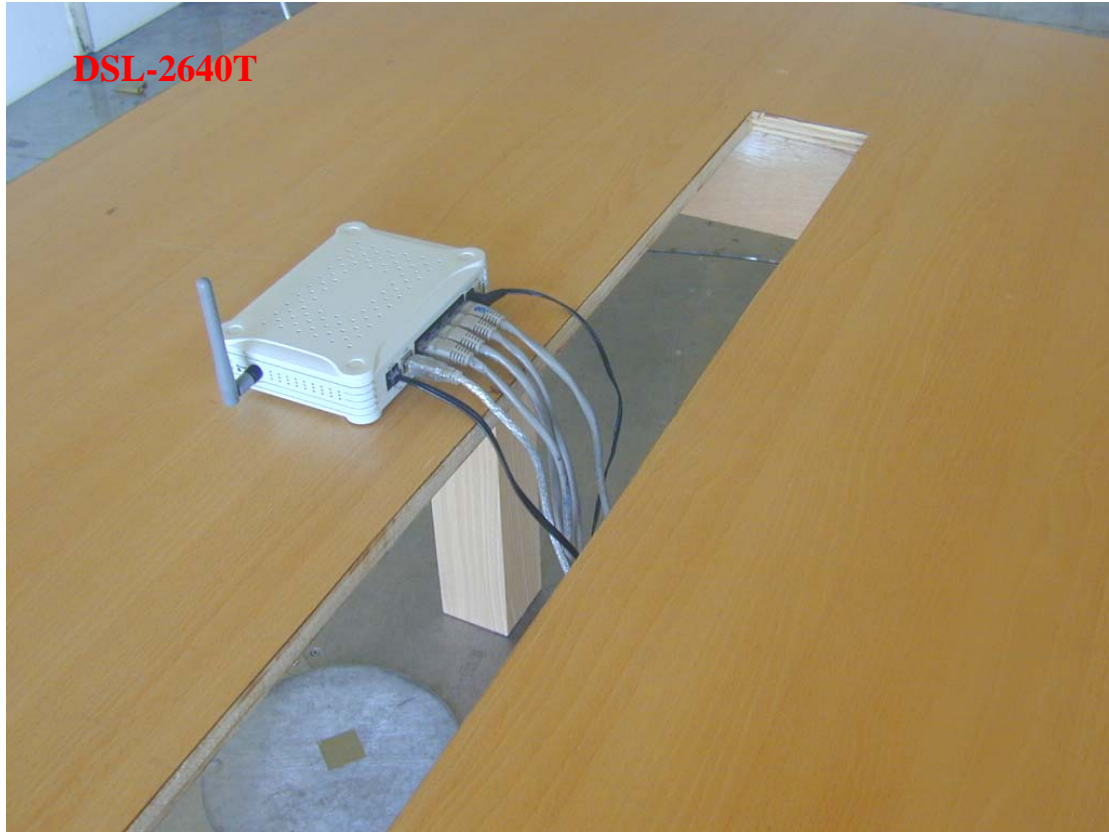
Photo 4: Radiated Emission Test Set-up
