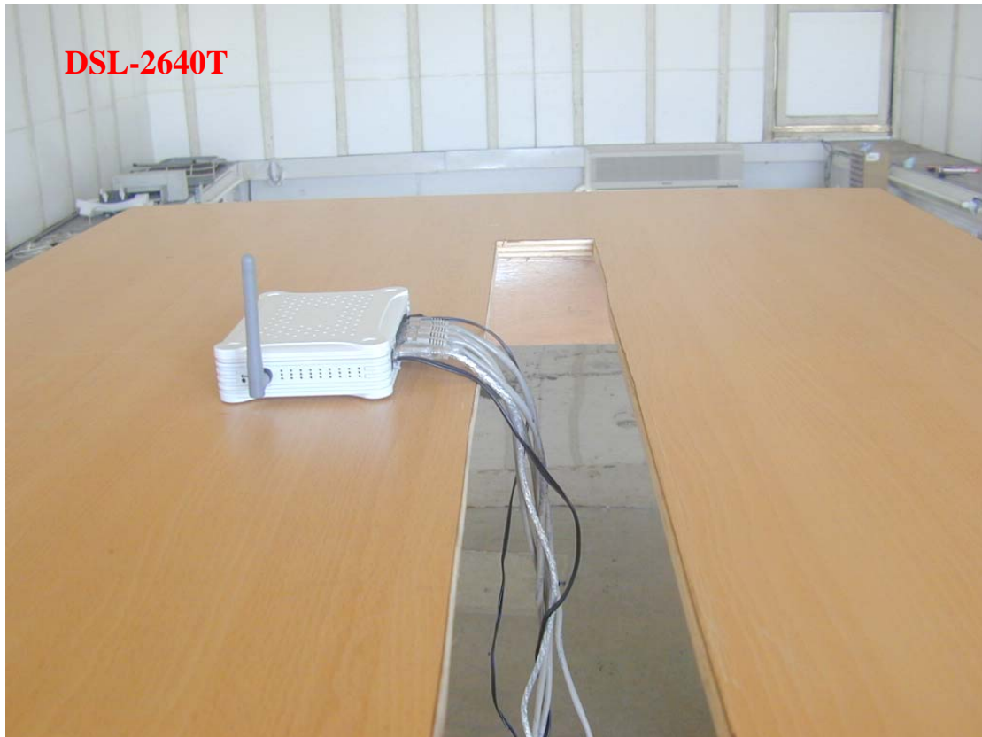
Photo 3: Radiated Emission Test Set-up
