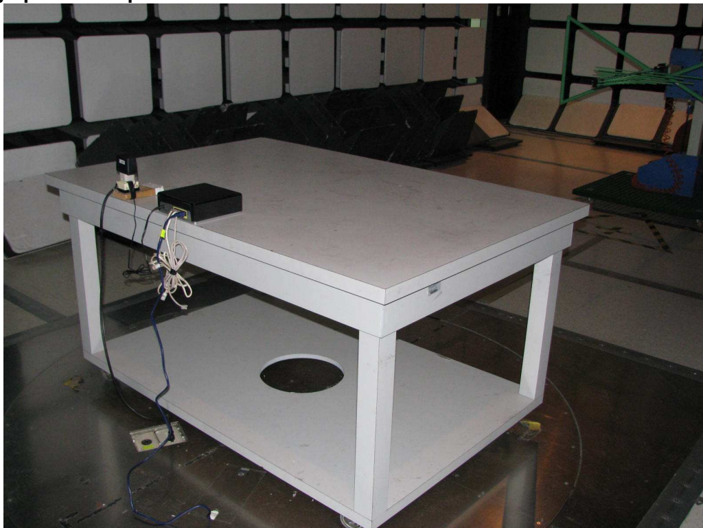
Photograph 2: Set-up for Radiated Emissions
