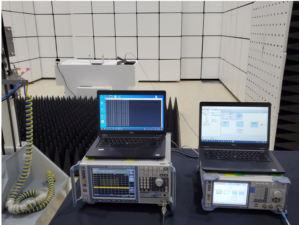
DFS Test Setup Photo: AP Mode
