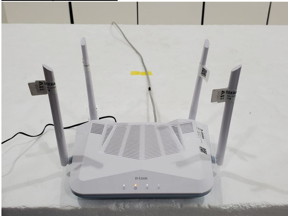
DFS Test Setup Photo: AP Mode
