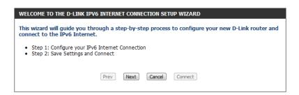
The router will try to detect whether its possible to obtain the IPv6 Internet connection type automatically. If this succeeds then the user will be guided through the input of the appropriate parameters for the connection type found.
