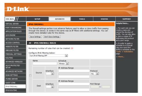
IP Address Range: Enter the source IPv6 address range in the adjacent IP Address Range field.
