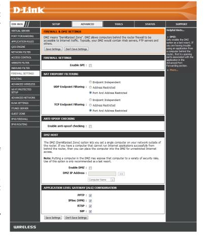
DMZ IP Address: Specify the IP address of the computer on the LAN that you want to have unrestricted Internet communication. If this computer obtains it's IP address automatically using DHCP, be sure to make a static reservation on the **Setup** > **Network Settings** page so that the IP address of the DMZ machine does not change.
