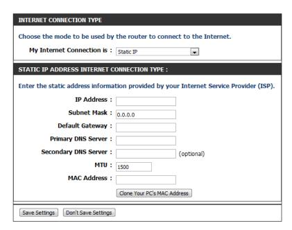
MAC Address: The default MAC Address is set to the Internet port's physical interface MAC address on the Broadband Router. It is not recommended that you change the default MAC address unless required by your ISP. You can use the **Copy Your PC's MAC Address** button to replace the Internet port's MAC address with the MAC address of your Ethernet card.
