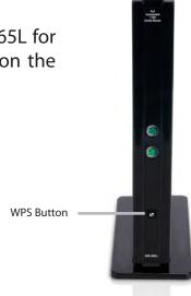
**Step 2** - Within 2 minutes, press the WPS button on your wireless client (or launch the software utility and start the WPS process).
