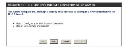
The router will try to detect whether its possible to obtain the IPv6 Internet connection type automatically. If this succeeds then the user will be guided through the input of the appropriate parameters for the connection type found.
