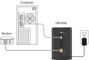
7. If you are connecting to a Broadband service that uses a dynamic connection (not PPPoE), you may be online already. Try opening a web browser and enter a web site. If a solid light indicates connection on the Internet port and the router can connect to the Internet. If the LED is orange, the connection is good but the router cannot connect to the Internet.
