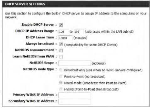
Enabling this option will cause the router to always broadcast its responses to all clients, thereby working around the problem, at the cost of increased broadcast traffic on the LAN.
