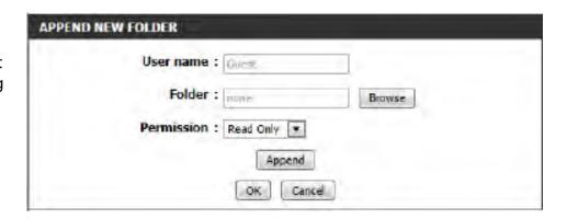
**Read Only** permission will only allow this account to read data stored on the USB storage device within the constrains of the access path specified. **Read/Write** permission will allow this account to read and write data to and from the USB storage device within the constrains of the access path specified.
