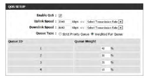
Queue Type: Here the user can specify the queue type used. When choosing the option Strict Priority Queue, the router will apply QoS based on the internal specification for the queue ID's listed. When choosing the option Weight Fair Queue, the router will apply QoS based on the user defined percentage in the Queue Weight column.
