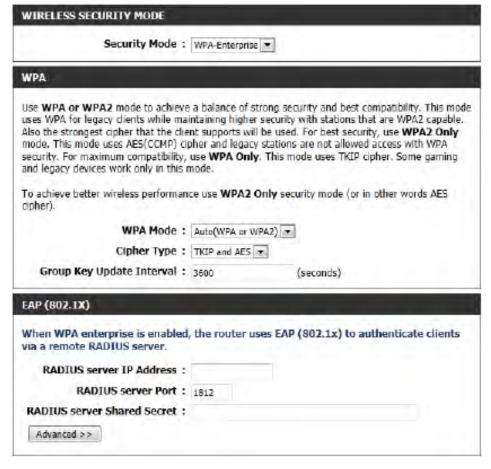
**RADIUS Server Port:** When the user chooses to use the EAP authentication framework, the RADIUS server's port number can be entered here.
