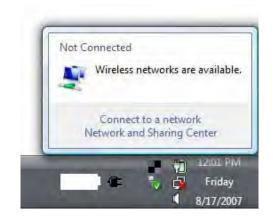
The utility will display any available wireless networks in your area. Click on a network (displayed using the SSID) and click the **Connect** button.
