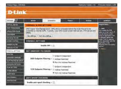
**DMZ IP Address:** Specify the IP address of the computer on the LAN that you want to have unrestricted Internet communication. If this computer obtains it's IP address automatically using DHCP, be sure to make a static reservation on the **Setup** > **Network Settings** page so that the IP address of the DMZ machine does not change.
