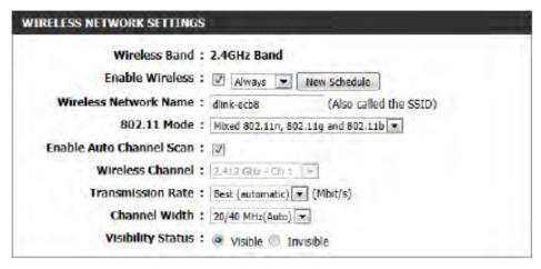
Wireless Network Name: The Service Set Identifier (SSID) is the name of your wireless network. Create a name using up to 32 characters. The SSID is case-sensitive. Enable Auto Channel
