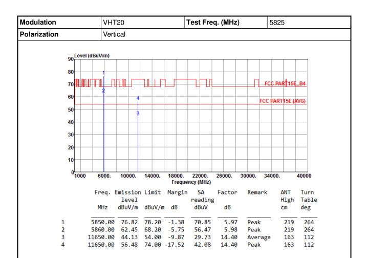
\*Factor includes antenna factor, cable loss and amplifier gain
