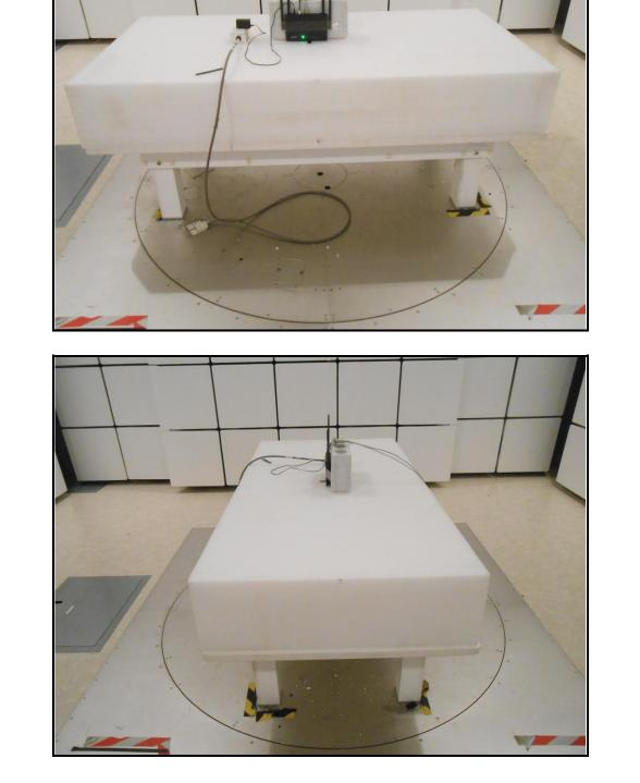
RADIATED EMISSION TEST (Below 1GHz)
