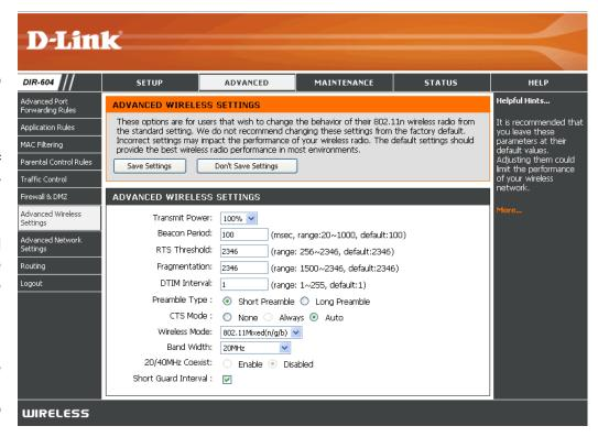
**Preamble** Select **Short** or **Long Preamble**. The preamble defines the length of the CRC block (Cyclic Redundancy Check is a common **Type:** technique for detecting data transmission errors) for communication between the wireless router and the roaming wireless network adapters. Note: High network traffic areas should use the **Short Preamble** type.
