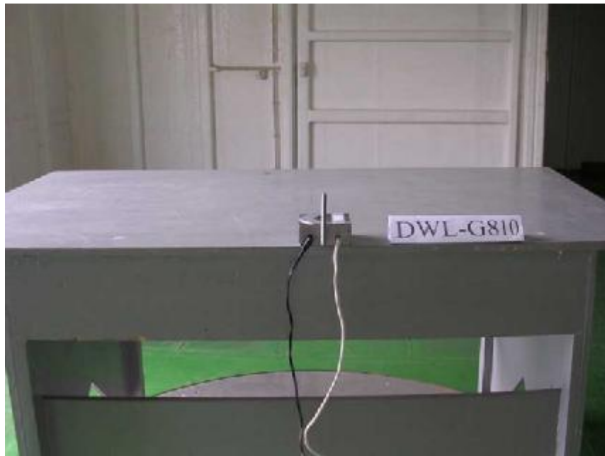
Photo 2: Radiated Emission Test Set-up
