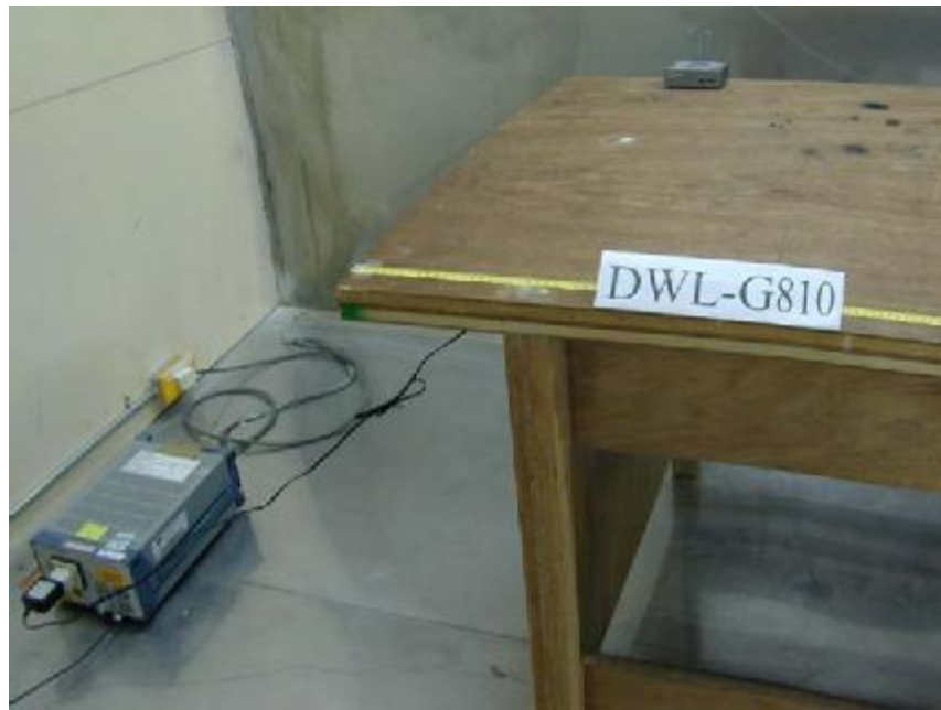
Photo 2: Conducted Emission Test Set-up
