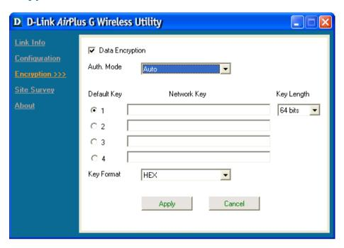
Data Encryption – Enable WEP encryption by clicking on the box.
