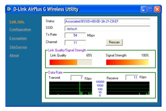
**Status:** Displays the MAC address of the access point that is associated with the DWL-G630.
