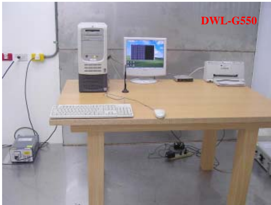
Photo 2: Conducted Emission Test Set-up
