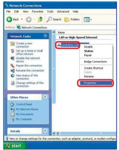
Assigning a Static IP Address in <u>Windows XP/2000</u>
