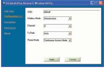
To communicate on the network all devices must have the same settings for the following properties:
