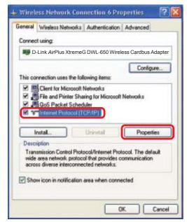
In the window below, select **Use the following IP Address**. Input your **IP Address and subnet mask**. (The IP Addresses on your network must be within the same range. For example, if one computer has an IP Address of 192.168.0.2, the other computers should have IP Addresses that are sequential, like 192.168.0.3 and 192.168.0.4. The subnet mask must be the same for all the computers on the network.)
