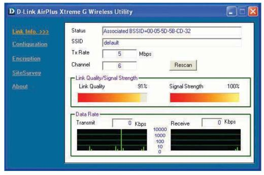
**Status:** Displays the MAC Address of the Access Point that is associated with the DWL-G520.
