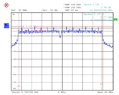
Modulation Type: OFDM-Turbo Mode(Channel 152) :
