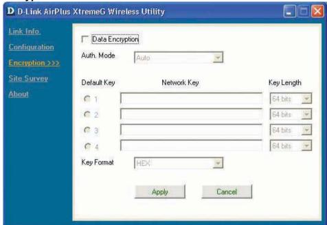
**Data Encryption** – enable Encryption by clicking on the box. Encryption is disabled as the default setting.
