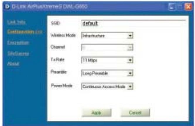
**To communicate on the network all devices must have the same settings for the following properties:**
