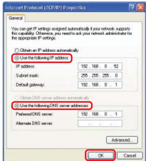
You have completed the assignment of a Static IP Address. (You do not need to assign a Static IP Address if you have a DHCP-capable Gateway/Router.)
