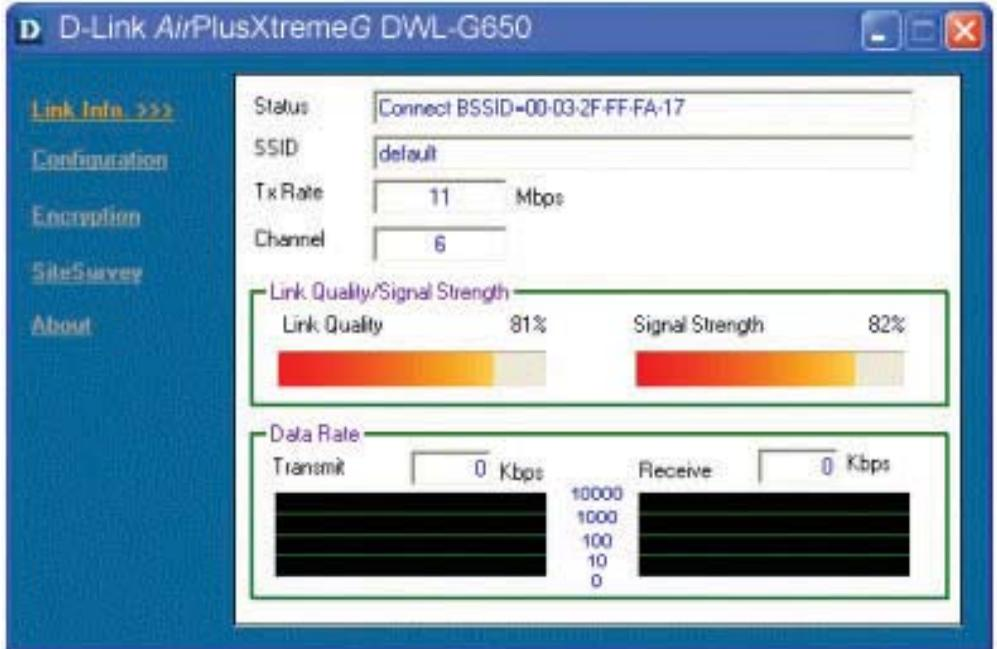
**Status:** Displays the MAC Address of the Access Point that is associated with the DWL-G650.
