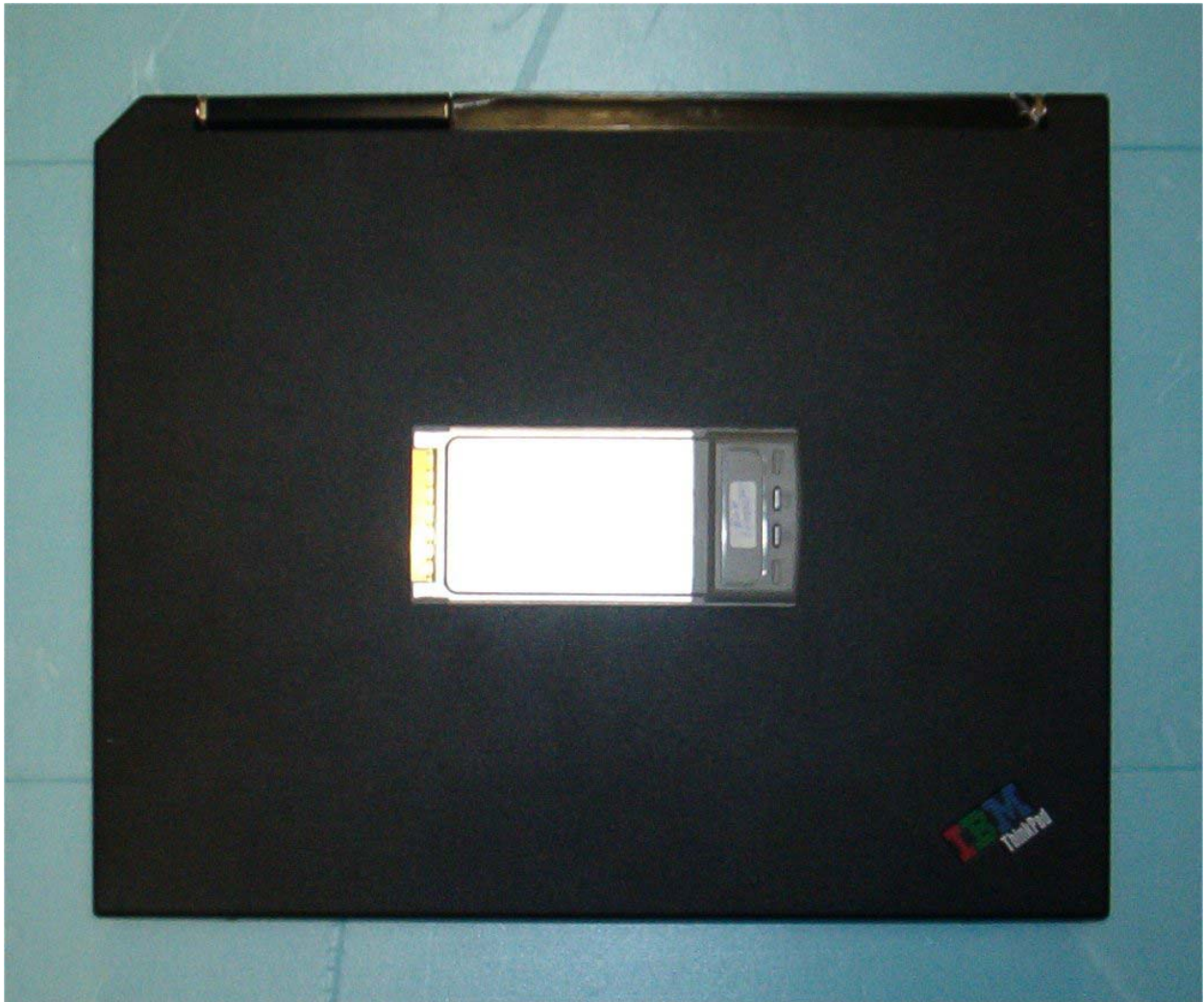
Fig. 2. A picture of the D-Link Model DWL-AG650 Cardbus Adapter placed on the IBM laptop computer.
