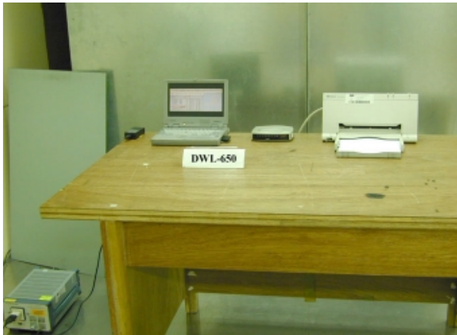
Photo 1: Conducted Test Set-up (front)
