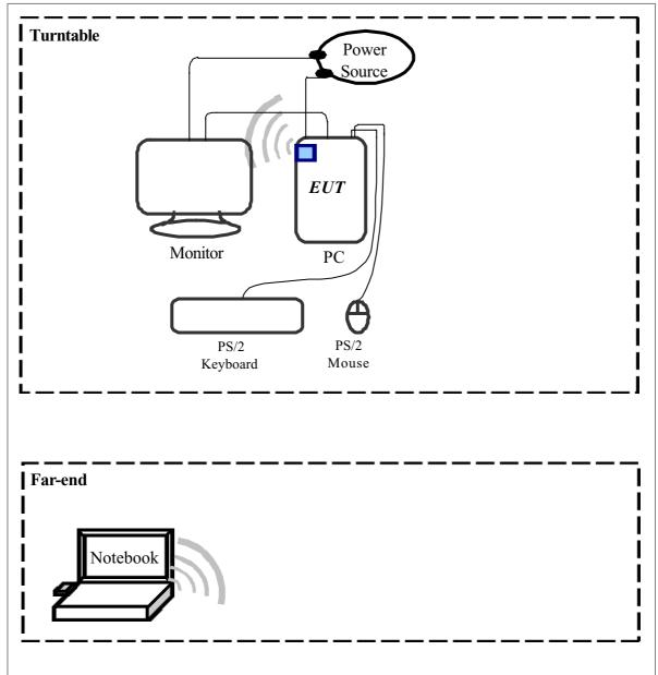
The tests below are carried out the EUT transmitter set at high power in TDD mode. The EUT is needed to force selection of output power level and channel number.
