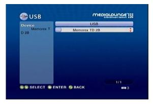
Use the selection arrows and press **ENTER** to select a USB thumbdrive for viewing. Depending on your photo display options, your files will either display in a list or as thumbnails. Press **ENTER** to display the image in a full screen and use the up and down selection arrows to navigate back and forward through your files. You can also select Auto Play in the setup menu and your files will automatically play when a card is inserted.
