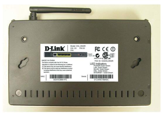
The Canada ID and DoC Label will be placed on the equipment as shown in the photograph below.
