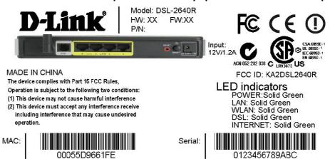
Wireless ADSL2+ Router Model No.: DSL-2640R FCC ID : KA2DSL2640R
