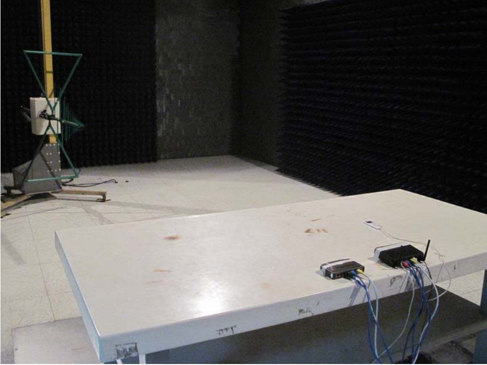
Description : Back View of Radiated Emission Test Setup for Below 1GHz
