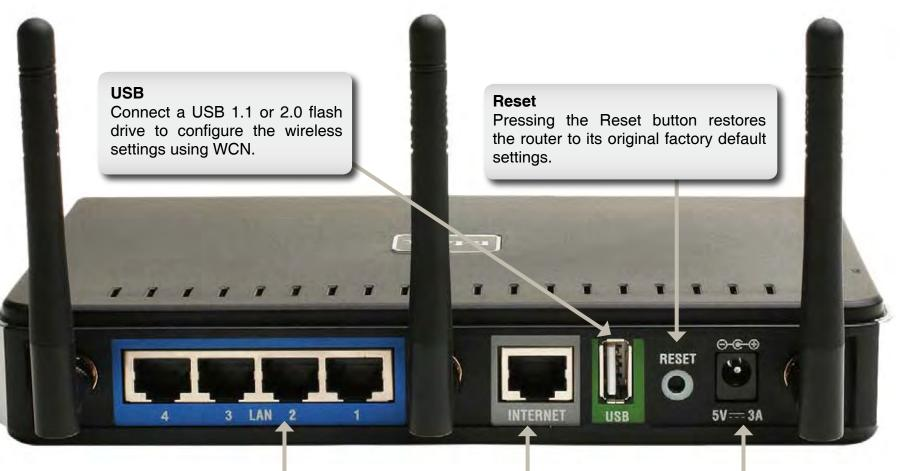
LAN Ports (1-4) Connect Ethernet devices such as computers, switches, and hubs.
