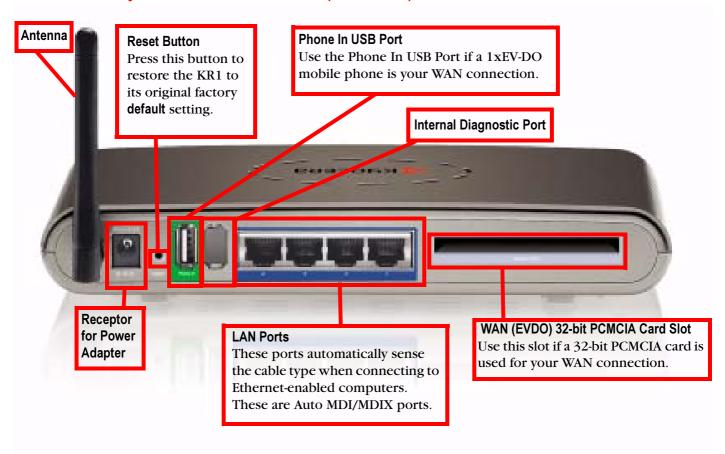
**Note:** The Kyocera KR1 Mobile Router contains two ports: a "Phone-In" USB Port, and a second internal diagnostic port. Please use *only* the "Phone In" USB port for your 1xEV-DO WAN connections.
