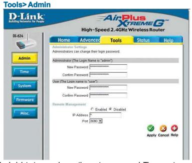
At this page, the DI-624 administrator can change the system password. There are two accounts that can access the Broadband Router's Web-Management interface. They are admin and user. Admin has read/write access while user has read-only access. User can only view the settings but cannot make any changes.
