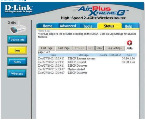
The Broadband Router keeps a running log of events and activities occurring on the Router. If the device is rebooted, the logs are automatically cleared. You may save the log files under Log Settings.
