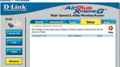
The wireless client table displays a list of current connected wireless clients. This table also displays the connection time and MAC address of the connected wireless client.
