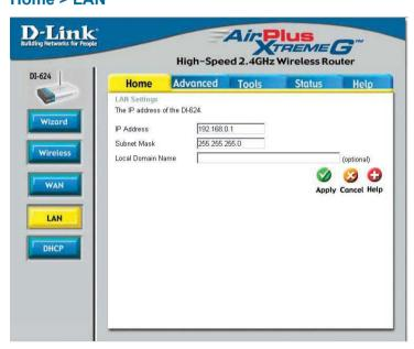
LAN is short for Local Area Network. This is considered your internal network. These are the IP settings of the LAN interface for the DI-624. These settings may be referred to as Private settings. You may change the LAN IP address if needed. The LAN IP address is private to your internal network and cannot be seen on the Internet.
