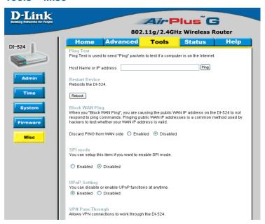
Ping TestThe Ping Test is used to send Ping packets to test if a computer is on the Internet. Enter the IP Address that you wish to Ping, and click **Ping**
