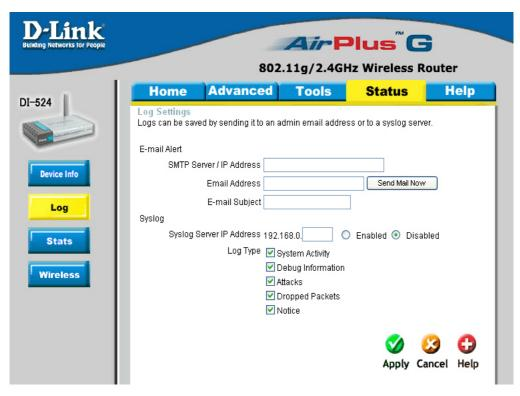
Not only does the Broadband Router display the logs of activities and events, it can setup to send these logs to another location.
