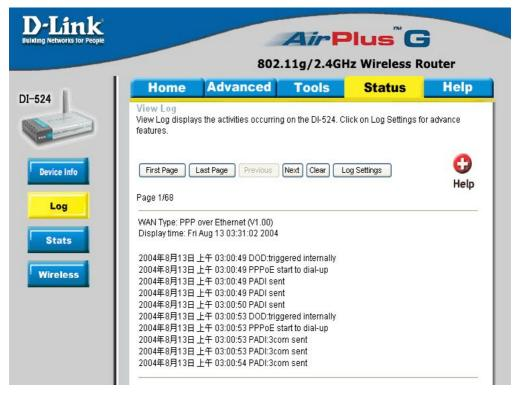
The Broadband Router keeps a running log of events and activities occurring on the Router. If the device is rebooted, the logs are automatically cleared. You may save the log files under Log Settings.
