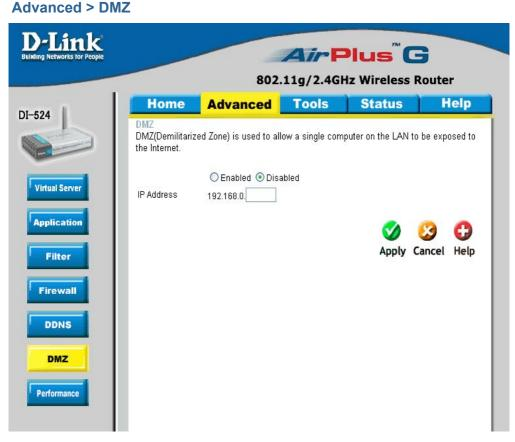
If you have a client PC that cannot run Internet applications properly from behind the DI-524, then you can set the client up for unrestricted Internet access. It allows a computer to be exposed to the Internet. This feature is useful for gaming purposes. Enter the IP address of the internal computer that will be the DMZ host. Adding a client to the DMZ (Demilitarized Zone) may expose your local network to a variety of security risks, so only use this option as a last resort.
