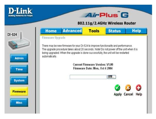
You can upgrade the firmware of the Router here. Make sure the firmware you want to use is on the local hard drive of the computer. Click on **Browse** to browse the local hard drive and locate the firmware to be used for the update. Please check the D-Link support site for firmware updates at http://support.dlink.com. You can download firmware upgrades to your hard drive from the D-Link support site.
