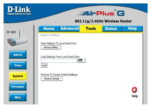
The current system settings can be saved as a file onto the local hard drive. The saved file or any other saved setting file can be loaded back on the Broadband Router. To reload a system settings file, click on **Browse** to browse the local hard drive and locate the system file to be used. You may also reset the Broadband Router back to factory settings by clicking on **Restore.**
