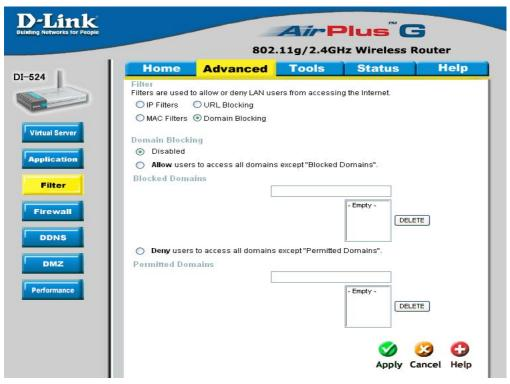
Domain Blocking is used to allow or deny LAN (Local Area Network) computers from accessing specific domains on the Internet. Domain blocking will deny all requests to a specific domain such as http and ftp. It can also allow computers to access specific sites and deny all other sites.
