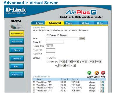
The DI-524 can be configured as a virtual server so that remote users accessing Web or FTP services via the public IP address can be automatically redirected to local servers in the LAN (Local Area Network).
