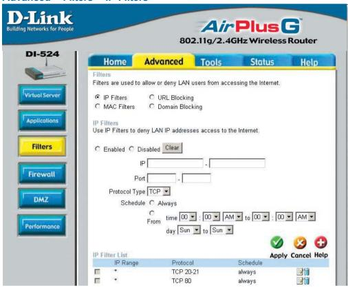
Filters are used to deny or allow LAN (Local Area Network) computers from accessing the Internet. The DI-524 can be setup to deny internal computers by their IP or MAC addresses. The DI-524 can also block users from accessing restricted web sites.
