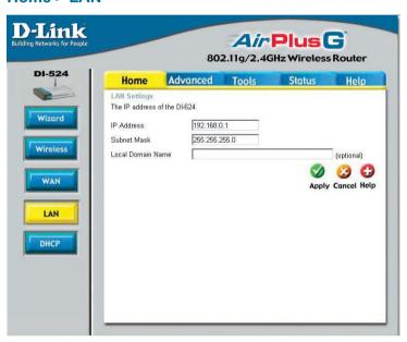
LAN is short for Local Area Network. This is considered your internal network. These are the IP settings of the LAN interface for the DI-524. These settings may be referred to as Private settings. You may change the LAN IP address if needed. The LAN IP address is private to your internal network and cannot be seen on the Internet.
