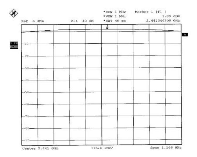
The Power (ERP) = Output power + cable loss + antenna gain = 1.89 dbm +1.3 db+ 1.9 dBi = 5.09 dbm
