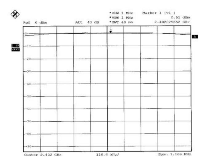
The Power (ERP) = Output power + cable loss + antenna gain = 0.51 dbm + 1.3 db + 1.9 dBi = 3.71 dbm
