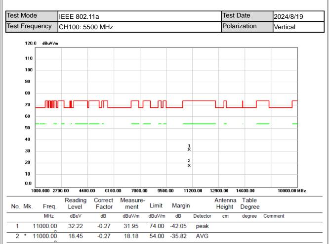
(1) Measurement Value = Reading Level + Correct Factor.
