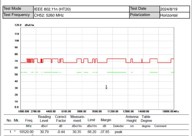
(1) Measurement Value = Reading Level + Correct Factor.
