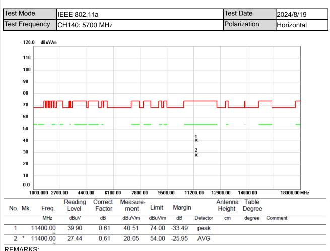
(1) Measurement Value = Reading Level + Correct Factor.
