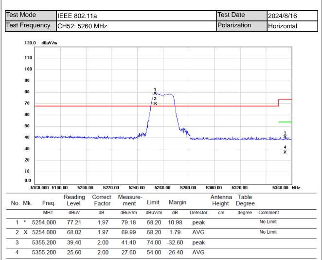
(1) Measurement Value = Reading Level + Correct Factor.
