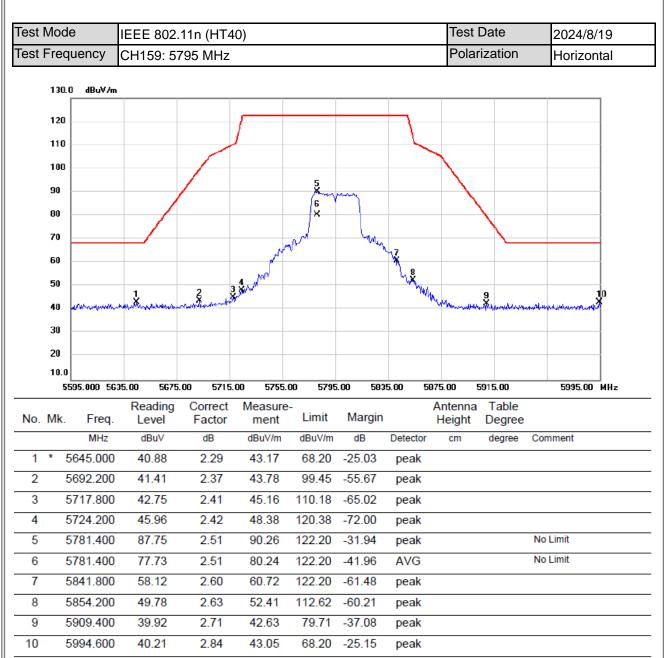
(1) Measurement Value = Reading Level + Correct Factor.
