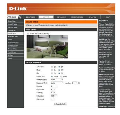
Exposure Mode: Changes the exposure mode. Use the drop-down box to set the camera for Indoor, Outdoor, or Night environments, or to Moving to capture moving objects. The Low Noise option will focus on creating a high-quality picture without noise. You can also create 3 different custom exposure modes. The Max Gain setting will allow you to control the maximum amount of gain to apply to brighten the picture.
