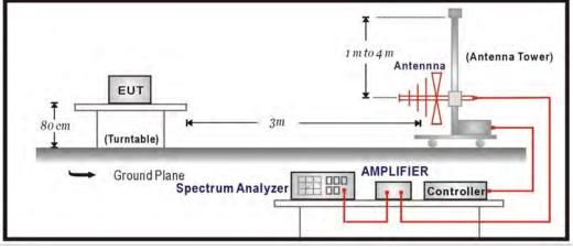
Above 1GHz Test Setup:
